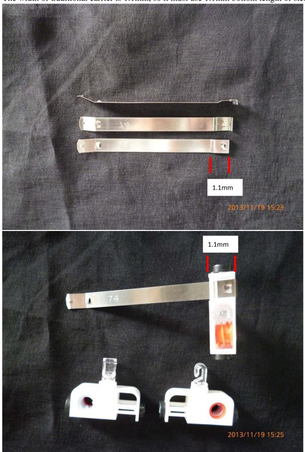
The carrier with removable hook is 0.8mm, so it must use 0.8mm bottom length of steel spacer.
